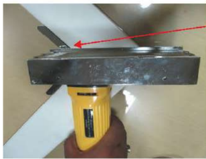
V Corner Cleaning Tool Model SP TL EL 05
